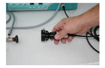
TV-Adapter connection to an endoscope
